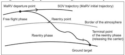
Fig. 1: The flight process of anti ground attack by MaRV
