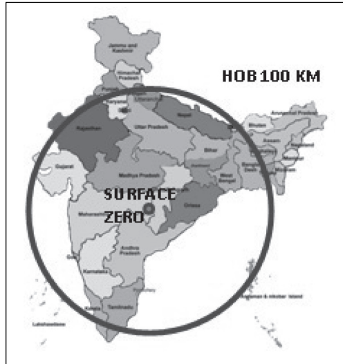
Fig 2: Coverage of Geographic Area by EMP Generated by a Nuclear Explosion at 100 km
