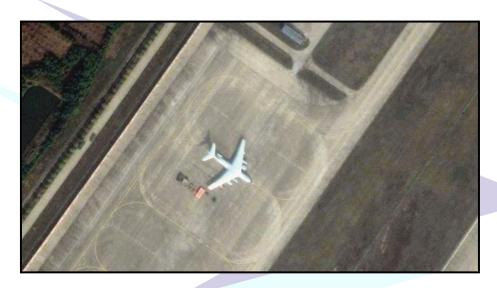
Satellite imagery of PLAAF IL-78 tanker aircraft parked at Wuhan-Paozhuwan airfield in Hebei province. Note the three refueling pods, one on each outer wing and one in the rear fuselage. Photo: IHS Jane's Defence Weekly, November 3, 2014, <a href="http://www.janes.com/article/45319/first-chinese-il-78-tanker-seen-at-plaaf-base">http://www.janes.com/article/45319/first-chinese-il-78-tanker-seen-at-plaaf-base</a>
