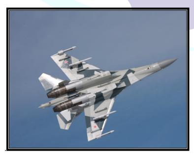
SU-35 showing its hard points. Each wing has four hard points – one on the wingtip and three under-wing stations. There are two hard points on the underside of the fuselage on the centreline and one under each engine. Photo: Sukhoi Company website
