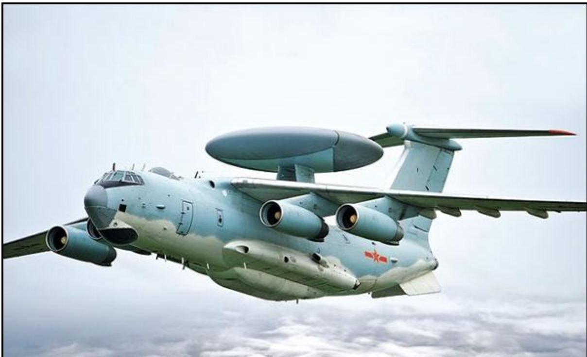
PLAAF AWACS on IL-76 platform. Note the triangle drawn on the lower side of the rotodome indicating the three sided planar array antenna inside. (Photo: Chinamil.com.cn/Ben Daochun)
