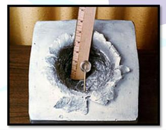
Figure 2: A 7 gram object (shown in centre) shot at 7 km/s (23,000 ft/sec) (the orbital velocity of the ISS) made this 15 cm (5 7/8 in) crater in a solid block of aluminium.<sup>11</sup>
