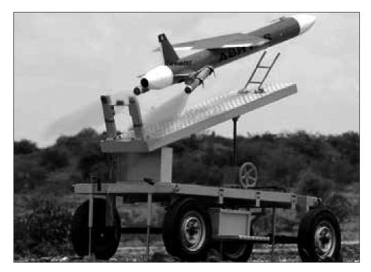
Fig 2: Abhyas Expendable Target Drone<sup>7</sup>
